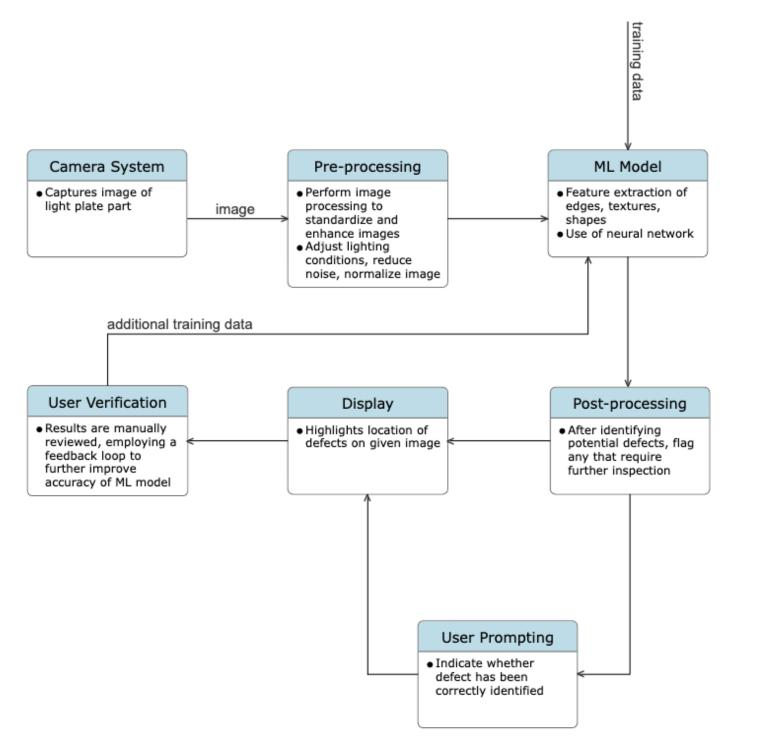
Our project uses computer vision to detect nonconformities on light plates of various sizes, meeting Safran's current inspection criteria and requirements. A block diagram of how we plan to execute and achieve this is shown in the block diagram.
